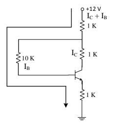
$\alpha = 0.99, V_{BE} = 0.7V, collector current is I<sub>C</sub>?$
