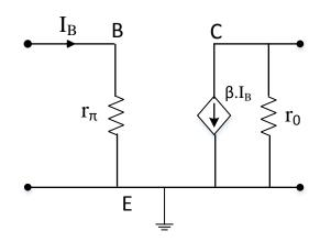
$$g_m = \frac{I_C}{V_i} = \frac{\beta I_B}{I_B r_\pi}$$
