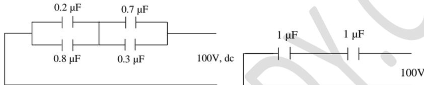
Each of parallel combination of capacitors is equal to  $1 \mu\text{f}$ . The voltage across each capacitor is 50 V. Charge on  $0.8 \mu\text{f} = 0.8 \times 50 = 40 \mu\text{c}$
