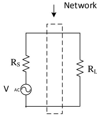
Maximum power is delivered to load when  $R_S = R_L = R$  If the network is lossless then
